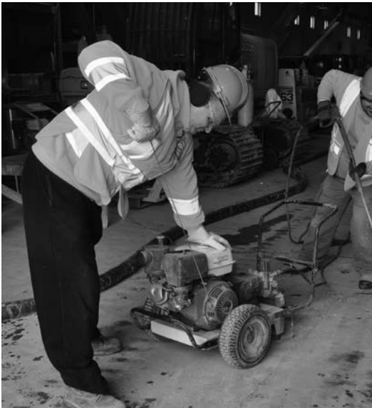
Used to clean concrete before re-sealing
