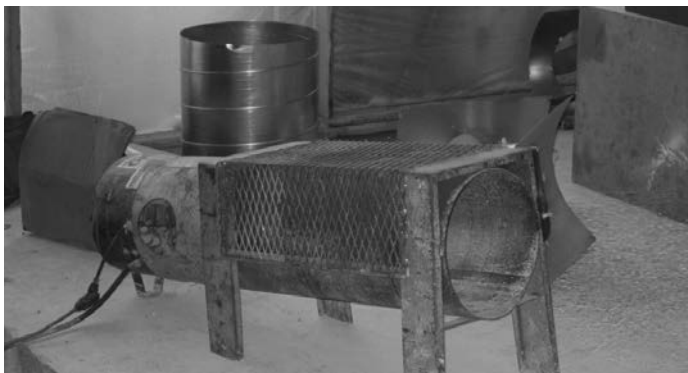
Figure 6-5: Open-flame Heaters Must Have Adequate Ventilation
