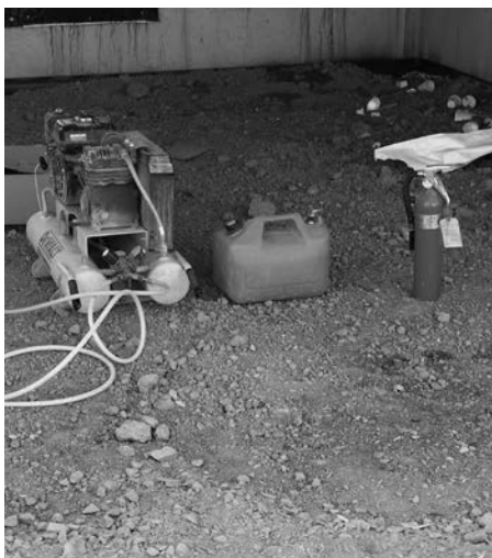
Used to power impact tools and other equipment powered by compressed air
